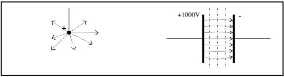
• Lines of equipotential are where the potential difference is the same in an electric field. In a uniform field the distance between lines of equipotential should be regular, so half way across the plate separation there will be half the voltage.
