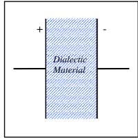
Capacitance is the measure of the size of a capacitor, defined by the surface area of the plates in the capacitor, and the plate separation. It also depend son the dielectric constant of the dielectric material which separates the two plates which make up a capacitor.
