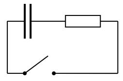
Since  $\sum V = \sum emf$   $0 = V_R + V$ From Q = CV and V = IR  $0 = \frac{Q}{C} + IR$ Since I = Rate of change of charge  $0 = \frac{Q}{C} + \frac{dQ}{dt}R$ Q = dQ = -
